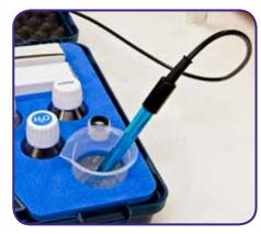
Measuring sample placed in a way that prevents accidental spills
