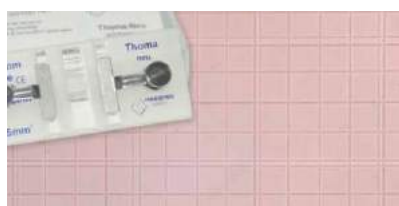
[2] WITH CLAMPS: similar to standard format but in this case the counting chamber is provided with a pair of clamps to hold the cover glass.
