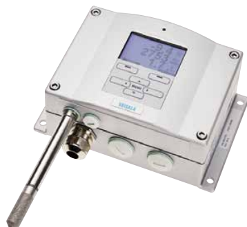
The DMT341 is made for installations in dry rooms where the entire dew point transmitter needs to be inside the dry space. The concept is easy to clean and suitable also for cleanrooms.
