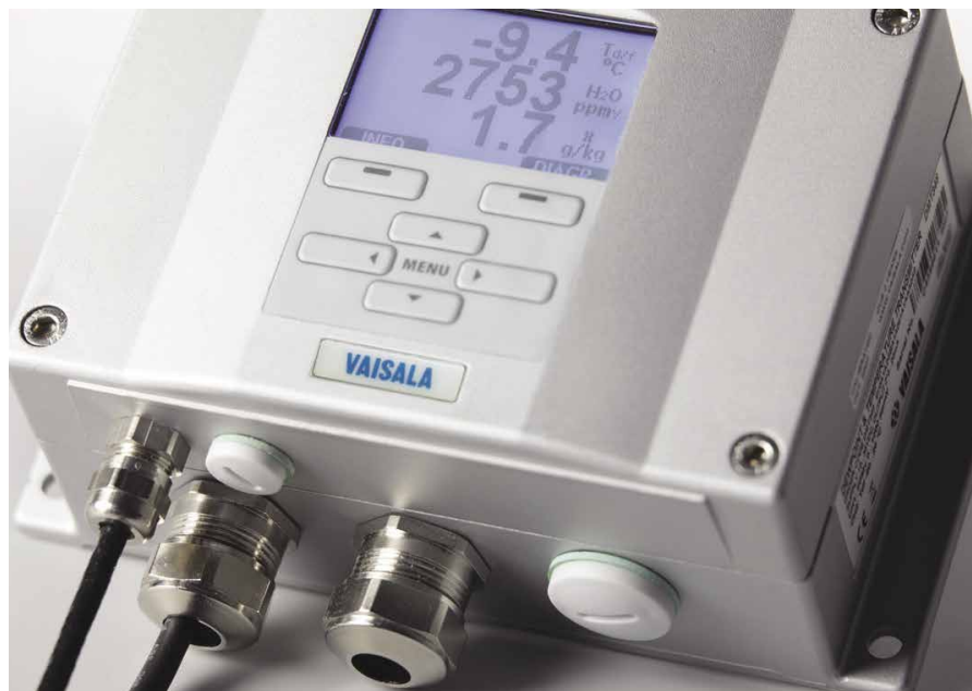
The display shows measurement trends, real-time data, and measurement history.
