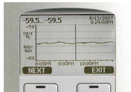
The display shows measurement trends, real-time data, and measurement history.
