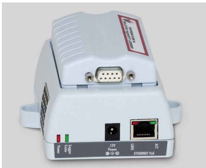
vNet Power over Ethernet interface with VL-2000 temperature and humidity logger.
