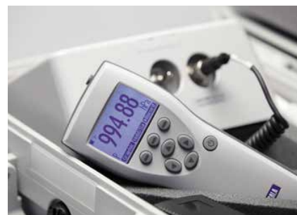
The MI70 hand-held indicator displaying the prevailing pressure in hPa
