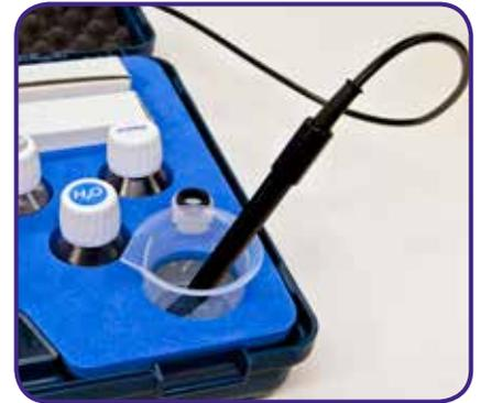
Measuring sample placed in a way that prevents accidental spills
